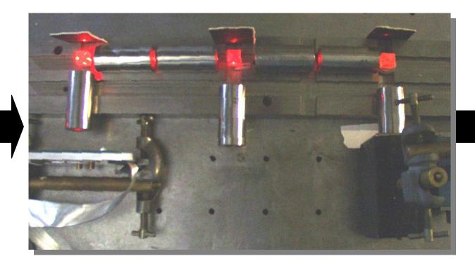
Proof-of-concept set-up to show polarisation routing used to send signal beams from VCSEL array to CCD cameras.
