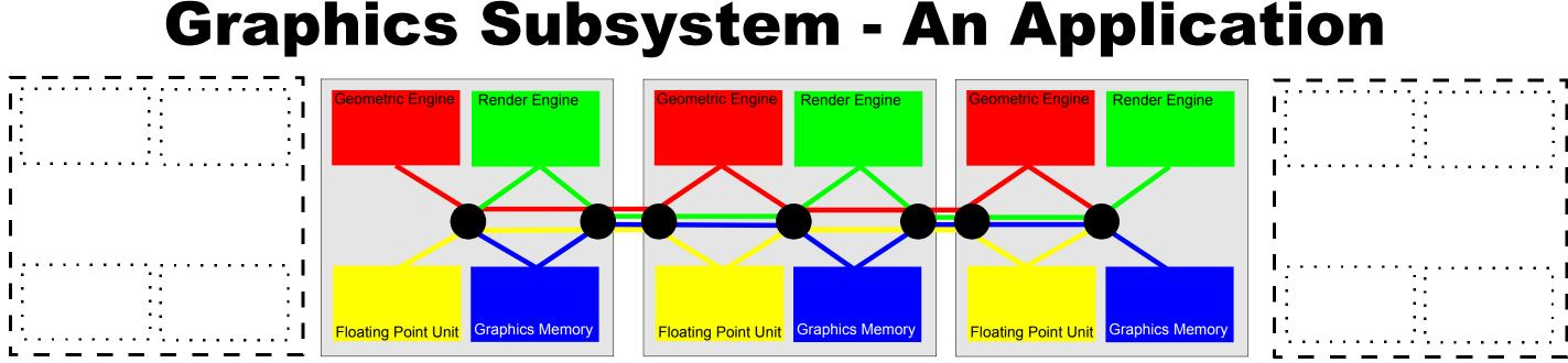
Processor Nodes are now the Geometric Engine, Render Engine, Floating Point Unit and other specialised processors. Interprocessor interconnect is also 'memory bus'.
