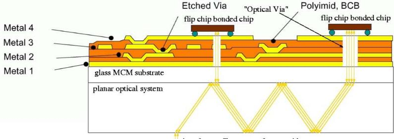
interface to fiber array of waveguide
