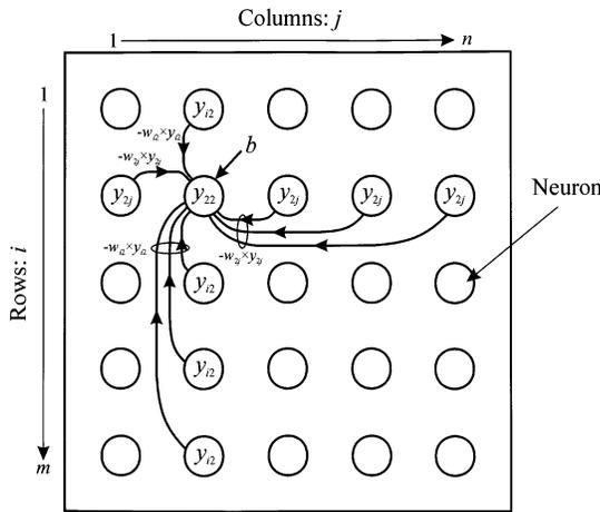
Fig. 2. Neural-network interconnection pattern mapped to an  $N = 5$  element crossbar switch. Neuron  $y_{22}$  receives inhibitory input from all other neurons in the same row and column. Note that  $m = n = N$ .
