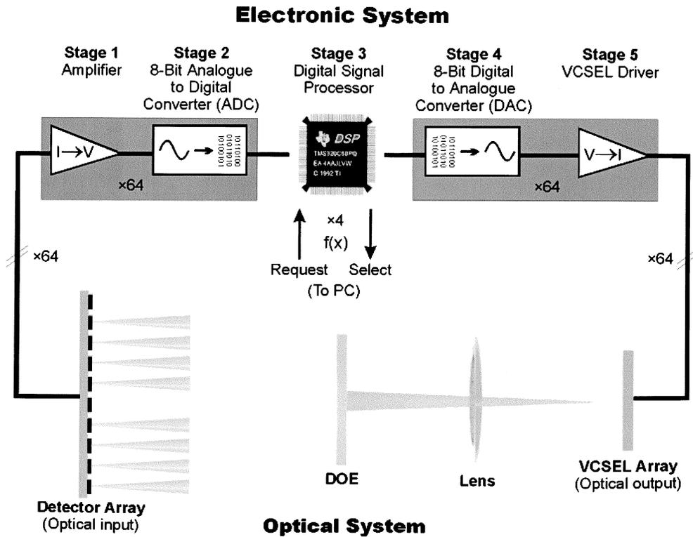
Fig. 3. Outline of the system currently under construction showing both optical and electronic pathways. This version is capable of routing eight input lines to eight output lines ( $N = 8$ , 64 channels in total).
