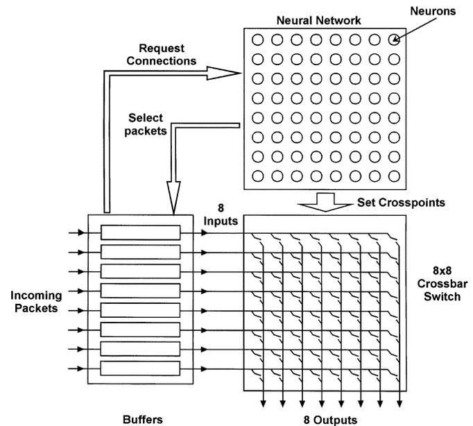
Fig. 1. Schematic of experimental neural-network crossbar switch controller. Based on the connections requested by incoming packets, the neural network chooses an optimal solution, sets the appropriate crosspoint switches, and then selects the chosen packets for transmission.
