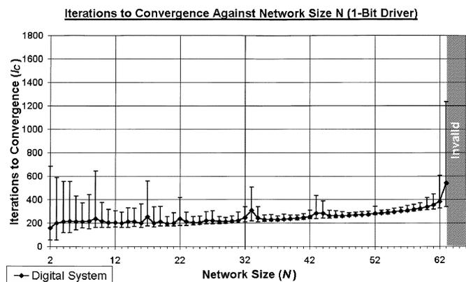
Fig. 6. Examination of the scalability of a digitally driven VCSEL system shows that convergence time is not greatly affected by network size. Average convergence times are indicated by the curve with error bars showing minimum and maximum outliers.
