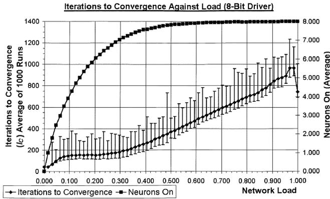
Fig. 7. Performance of an 8-bit analog-like driver under varying load conditions. Averages indicated by the curve with error bars showing minimum and maximum outliers.
