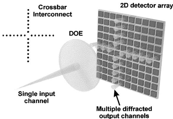
Fig. 4. Interconnect pattern formed by a single input channel incident on the DOE. All detectors and thereby associated neurons in the same row and column receive an inhibitory signal from incident light: thus the missing zeroth order—self inhibition would prevent network evolution.
