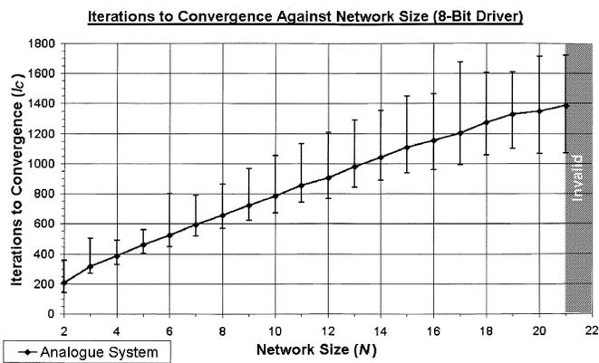
Fig. 5. Scalability of an 8-bit (analog like) driver which has a linear increase in the average number of iterations required as  $N$  increases. Average convergence times are indicated by the curve with error bars showing minimum and maximum outliers.
