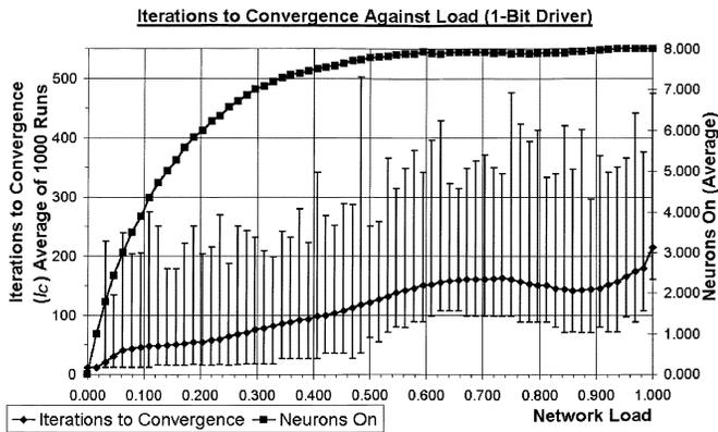
Fig. 8. Performance of a digitally driven network under varying load conditions. Averages indicated by the curve with error bars showing minimum and maximum outliers.
