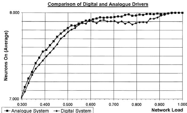
Fig. 9. Comparison of quality of solution between digital and analog systems. Averages indicated by the curve.
