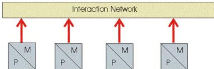
Each processor has its own local memory. MIMD's of this type are often called multi-computers. They can be on the same PCB or can use a LAN but for either type a high bandwidth interconnect is needed. This architecture is cost effective if most memory access is to local memory. As memory is local the system can be optimised for low memory latency.
