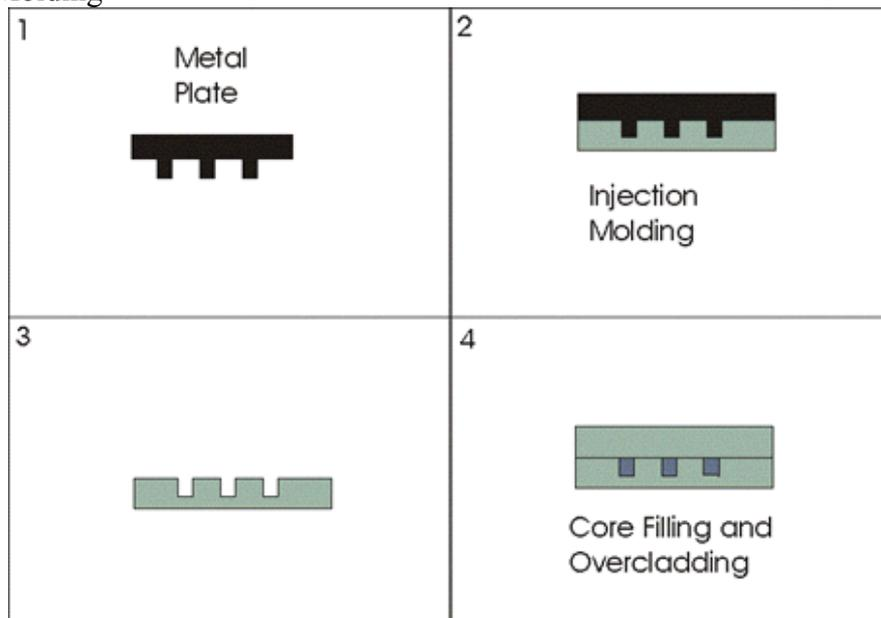
[26], [28] shows a buried waveguide by the injection molding technique. A metal imprint of the waveguides is transferred to an injection molding machine. The metal is removed and the waveguide structure is defined by grooves. The grooves are then filled by polymer to create the waveguide core. A polymer plate is then pressed onto the waveguides. This removes any excess liquid and protects the waveguides. The waveguides are then cured.
