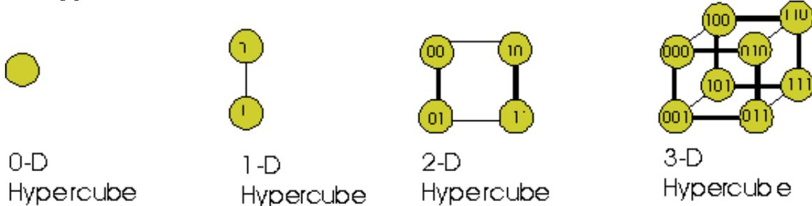
A hypercube is a multidimensional mesh of processors with exactly 2 processors in each dimension. The binary representation of each processor is included in the diagrams above. Each processor is connected to another only if their binary representations differ by only one bit position. In a  $d$ -dimensional hypercube each processor is connected to  $d$  other processors. Other parameters are given in [14].
