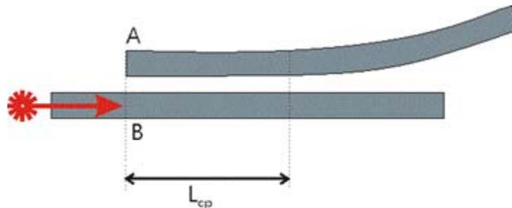
The evanescent field from waveguide B excites a mode in waveguide A. How much power is transferred is dependent on the proximity and length of the coupling region.
