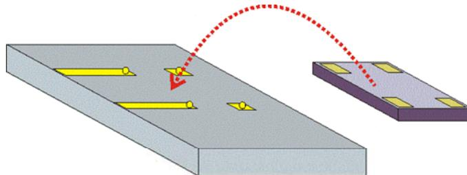
Solder bump flip chip was developed by IBM in 1960. The technology was developed because it was realised that compared to the traditional wire bonding techniques it would yield
