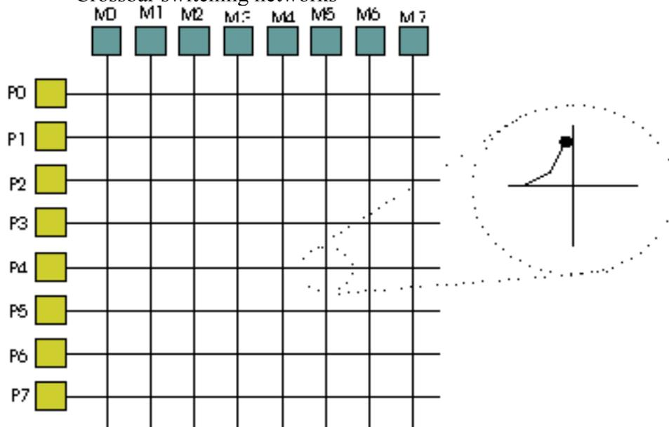
This consists of a grid of switching elements so that any processor can access any memory bank. The number of memory banks must be at least equal to the amount of processors otherwise some processors may not be able to access any memory. As the amount of processors becomes large, the switching network becomes unpractical due to the size of the switching network required.
