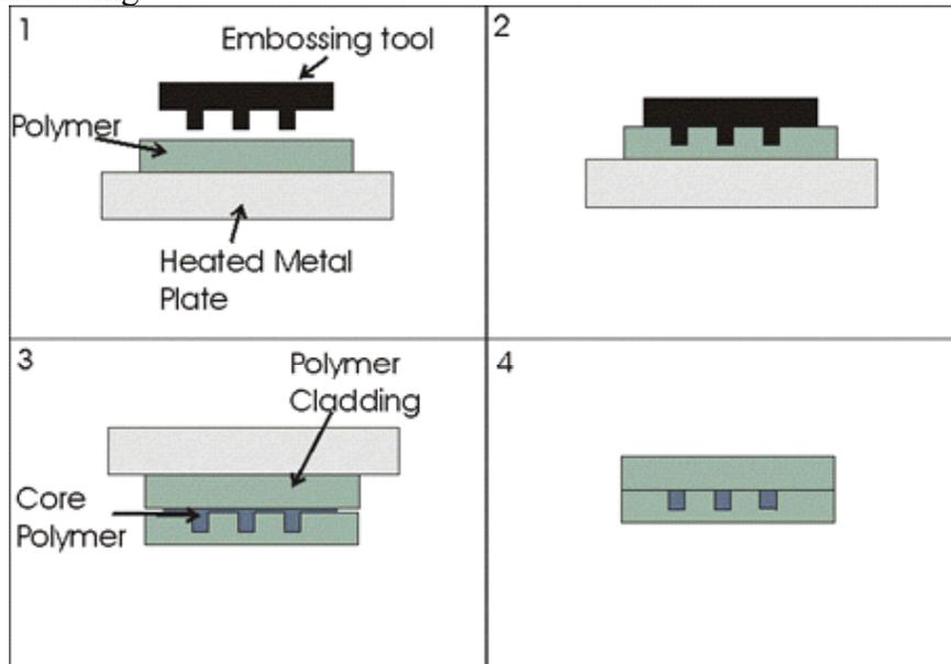
[27] shows an embossing technique for polymer waveguides. A metal masterform is used to emboss the waveguides as grooves into the polymer foil. The grooves are then filled with liquid core polymer, which is hardened and then covered with cladding. The thin polymer foil containing the optical layer is then laminated onto the PCB.
