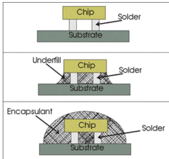
The underfill / encapsulant is to improve reliability by reducing stress. The processes of flip chip will now be considered.
