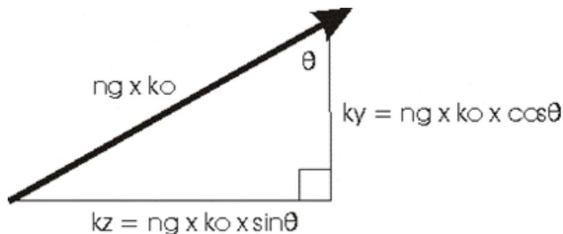
The portion of the propagation constant travelling in the z direction is then calculated by:
