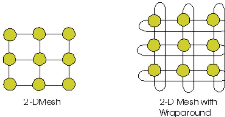
The mesh is an extension of the linear array to 2 dimensions. Each processor has a direct link to four other processors. For extra connectivity the processors at the edge can be connected by wraparound connections.
