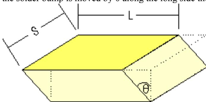
$$\begin{aligned}\Delta A_L &= 2S\left(\frac{H}{\cos\theta}\right) - 2SH \\ &= 2SH\left(\frac{1}{\cos\theta} - 1\right)\end{aligned}$$
