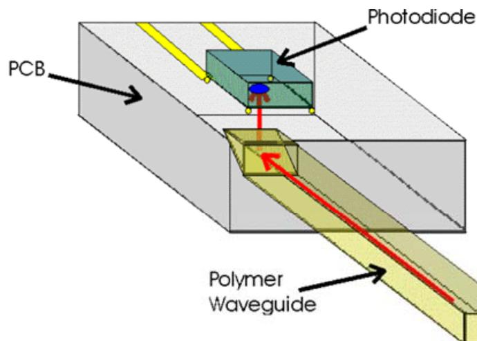
This is best explained by example. To align the PD, light would be launched into the waveguide and the PD moved into such a position that the photocurrent is maximised. This method is time consuming and requires dedicated machinery.
