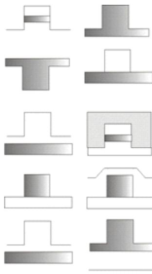
The grey area shows where the region where the light is being guided. The structures can be formed in all standard substrates by etching, doping and growing. The following sections will concentrate on a rib waveguide.
