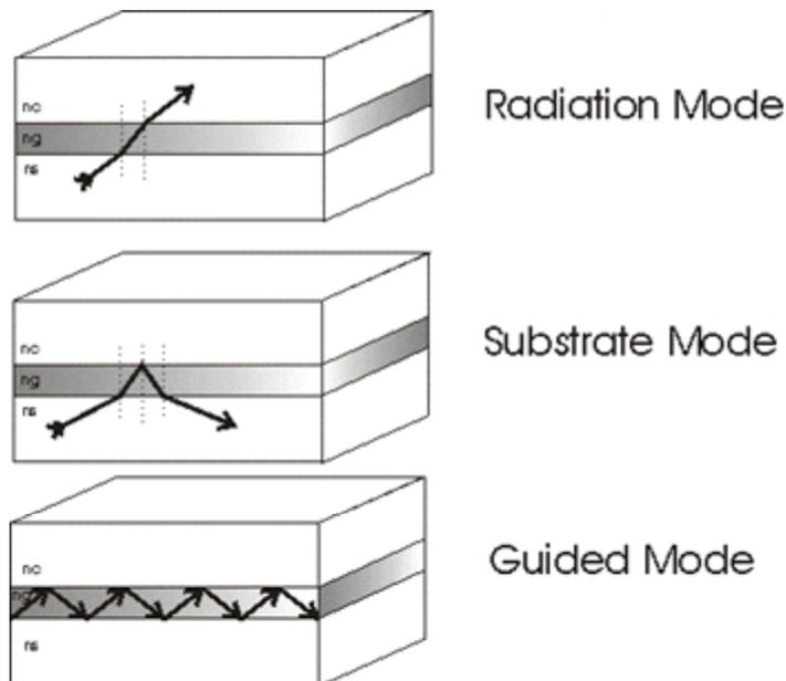
There are also other solutions as described in [36] that allow for leaky modes that are guided but diverge at infinity. A description will not be given here but it should be noted when designing a system. This section has given a quick overview of the EM theory of slab waveguides. The ideas outlined here can be extended to a 2-d confined wave in a guiding layer.
