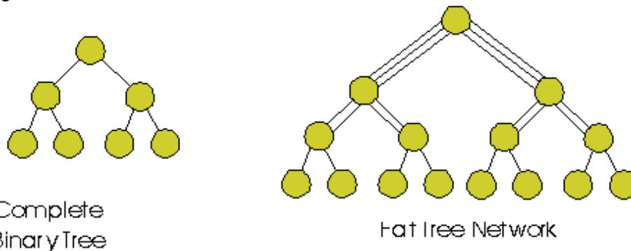
In the tree network there is only one path between any pair of processors. Linear array and star network are special cases of tree network. At higher levels of the tree there is a communication bottleneck. This can be solved by adding extra links higher in the tree.
