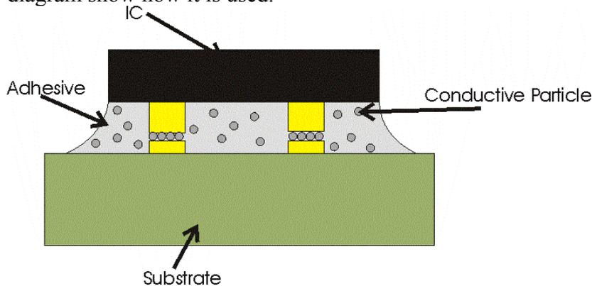
The ACF is first laid on the substrate. The chip is then aligned and the adhesive cured. A good contact assumes that the density and distribution of the conducting particles is such that when the IC and substrate are in contact it is assured that there will be enough particles between the pads. One shortcoming of this method is that the amount of particles between the pads cannot be controlled implying the possibility of some poor electrical contacts.
