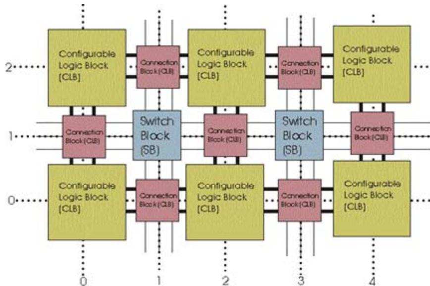
The switching blocks and connection blocks are user definable, meaning that the chip can be reconfigured as to what its functionality is. This gives the FPGA its usefulness [63].
