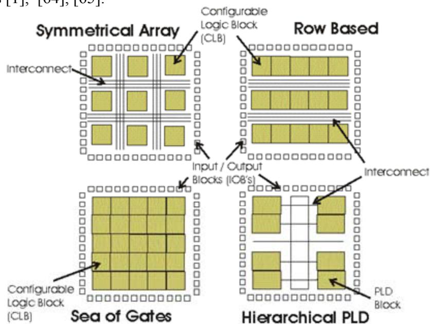
An FPGA consists of logic blocks with interconnections in between. As shown in the next diagram there are switching blocks and connection blocks on these interconnections.
