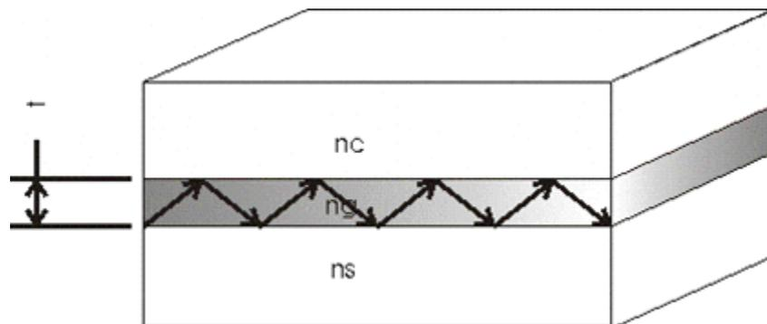
By considering this diagram it can be seen that if the wavefronts from A and B are not in phase then destructive interference will occur along the waveguide and the light will no longer propagate.
