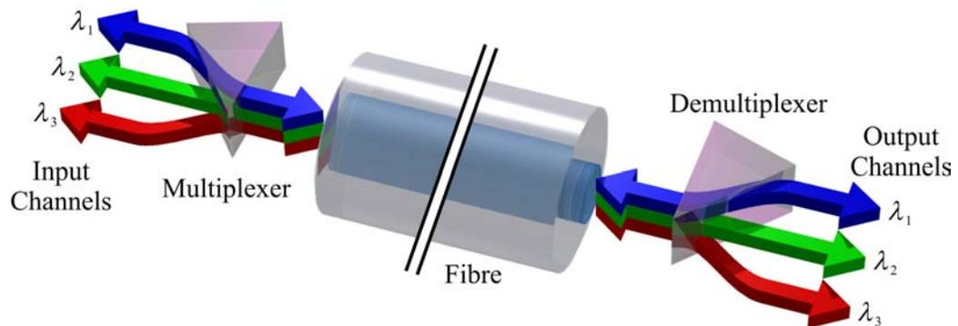
**Figure 12: Wavelength Division Multiplexing**
