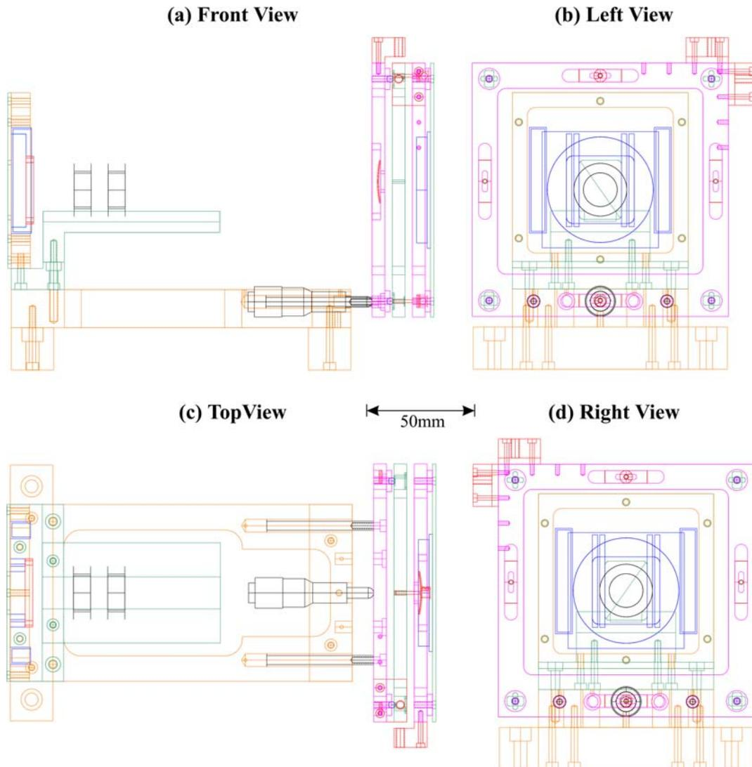
**Figure 101: Baseplate Schematics**
