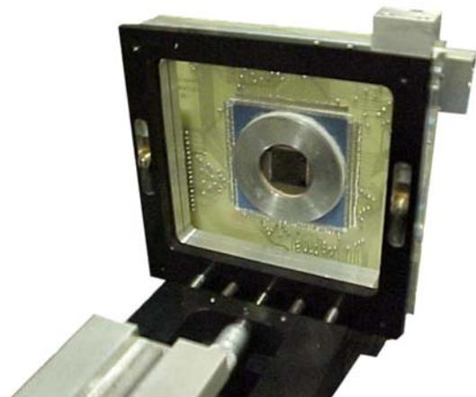
**Figure 106: Detector PCB Layout and Mount**
