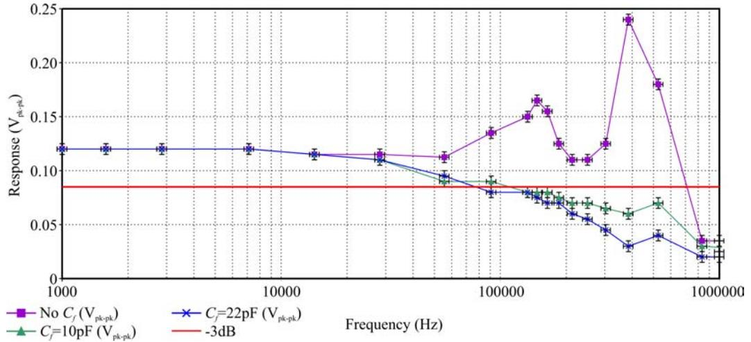
**Figure 118: Transimpedance Amplifier Measured Bandwidth**
