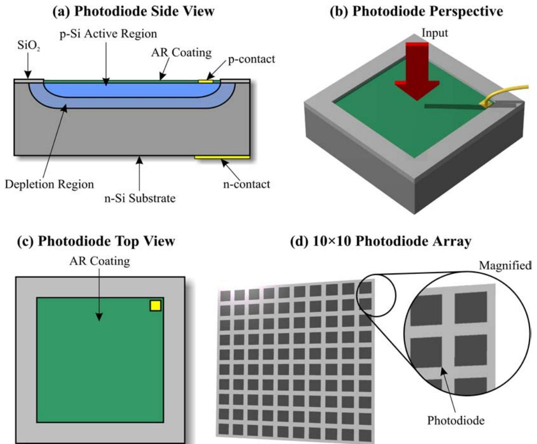
**Figure 30: Photodiode Detector**
