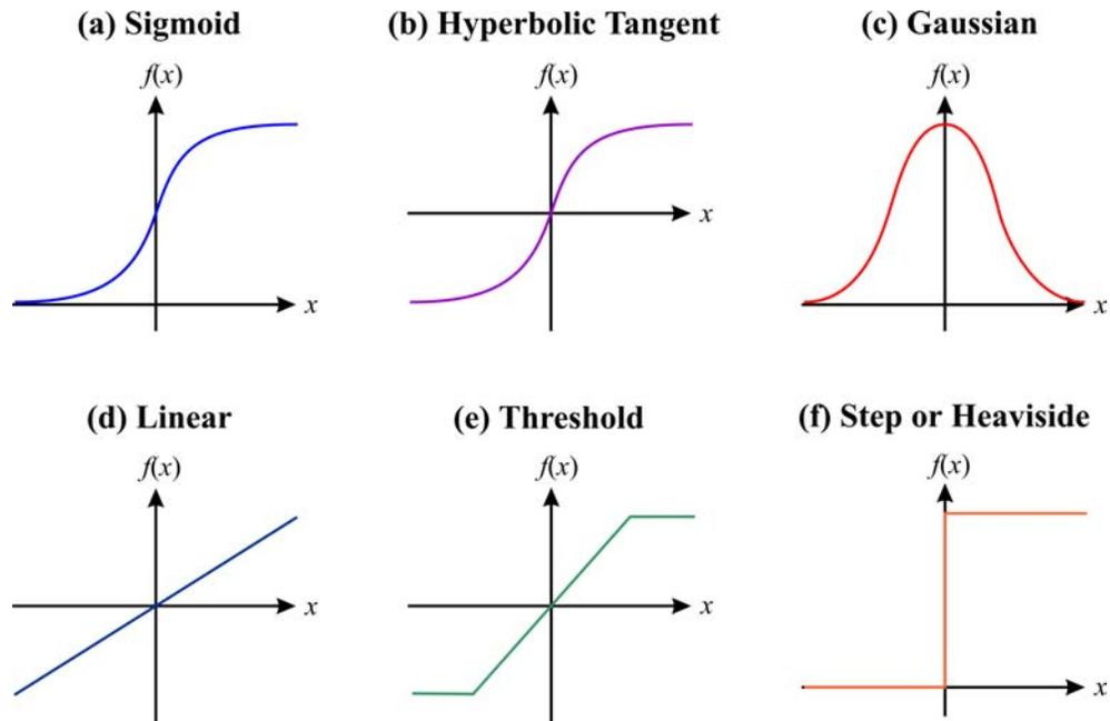
**Figure 48: Sample Transfer Functions**
