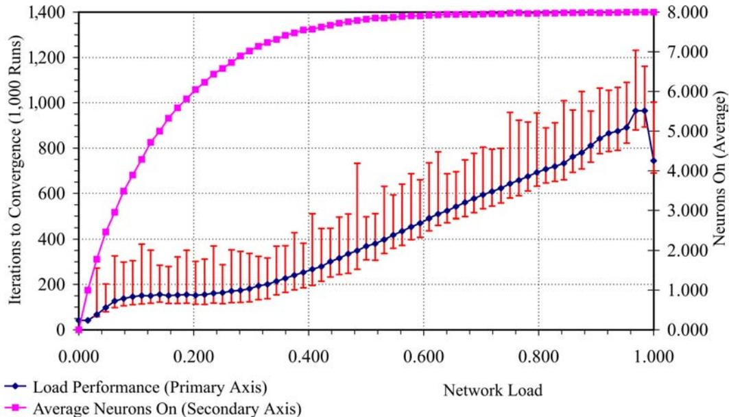
**Figure 67: Effect of Load on Iterations to Convergence with  $Q_{DAC}=8$**
