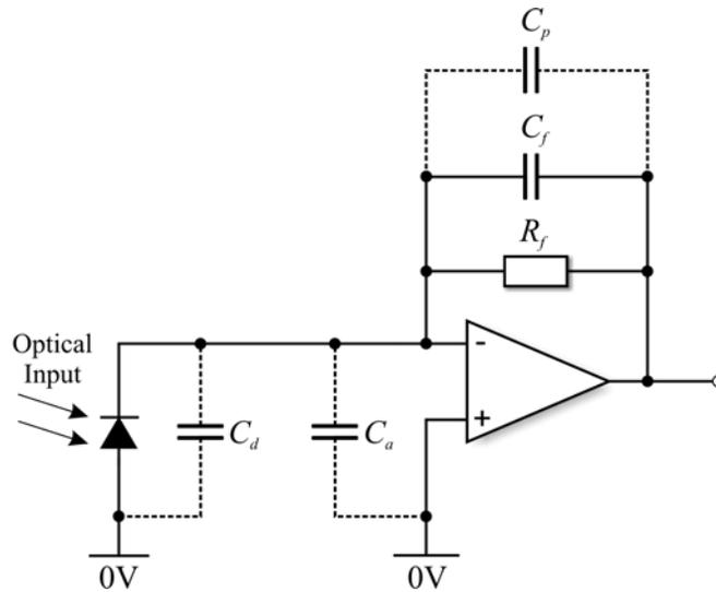
**Figure 34: Operational Amplifier Bandwidth Limitations**
