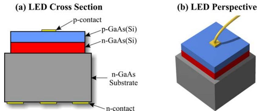
**Figure 26: Near Infrared Light Emitting Diode (LED)**
