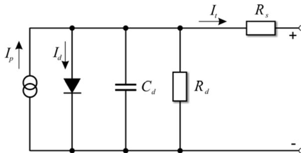
**Figure 31: Photodiode Electrical Model**
