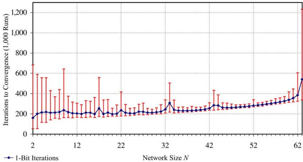
**Figure 66: Effect of Network Size  $N$  on Iterations to Convergence with  $Q_{DAC}=1$**
