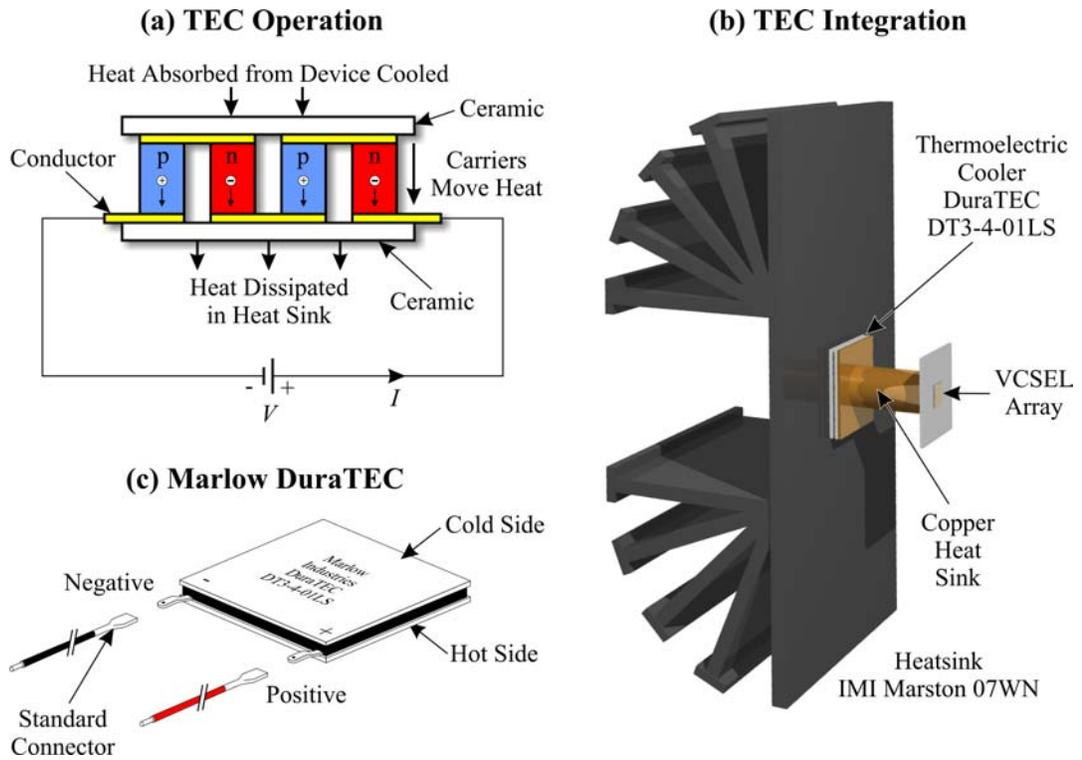
**Figure 112: DuraTEC DT3-4-01LS Thermoelectric Cooler**
