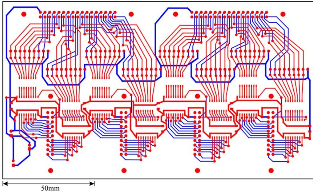
**Figure 98: Digital VCSEL Driver Module PCB Layout**
