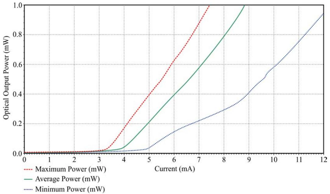
**Figure 73: Lase-Array SN 2640 VCSEL Optical Output Power Characteristics**
