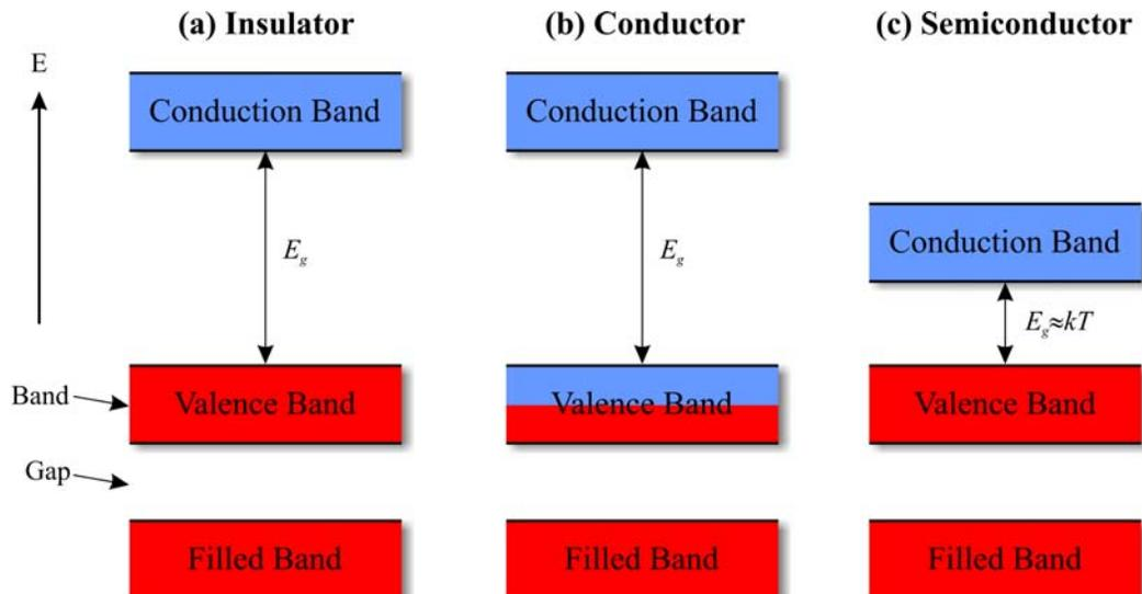
**Figure 23: Energy Levels in a Lattice**
