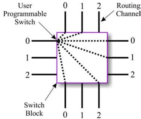
**Figure 127: Switch Block**
