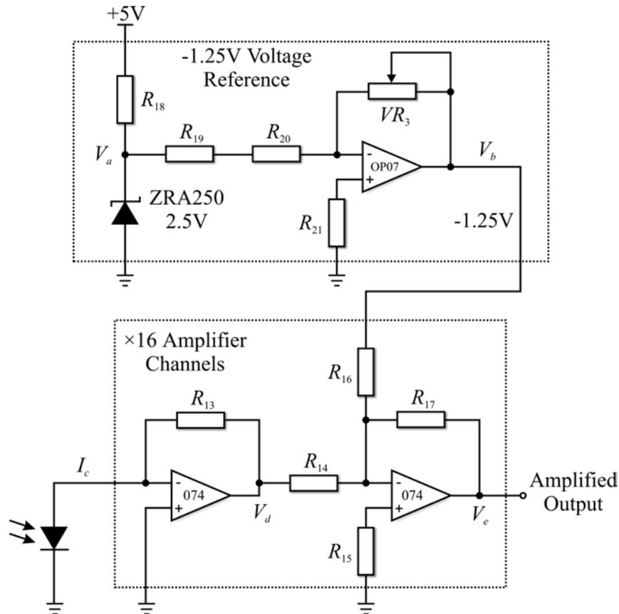
**Figure 114: Transimpedance Amplifier Circuit Diagram**
