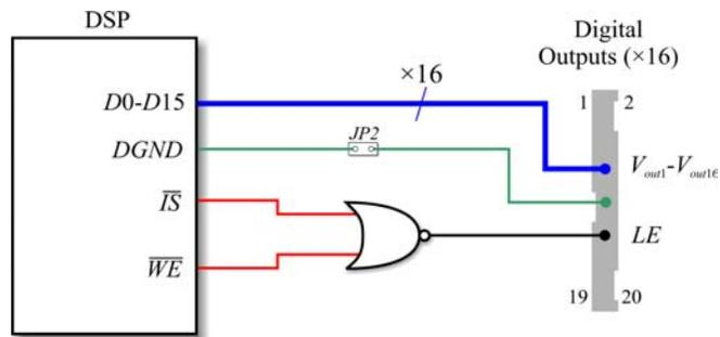
**Figure 94: DSP to Digital Output Interface Circuitry**
