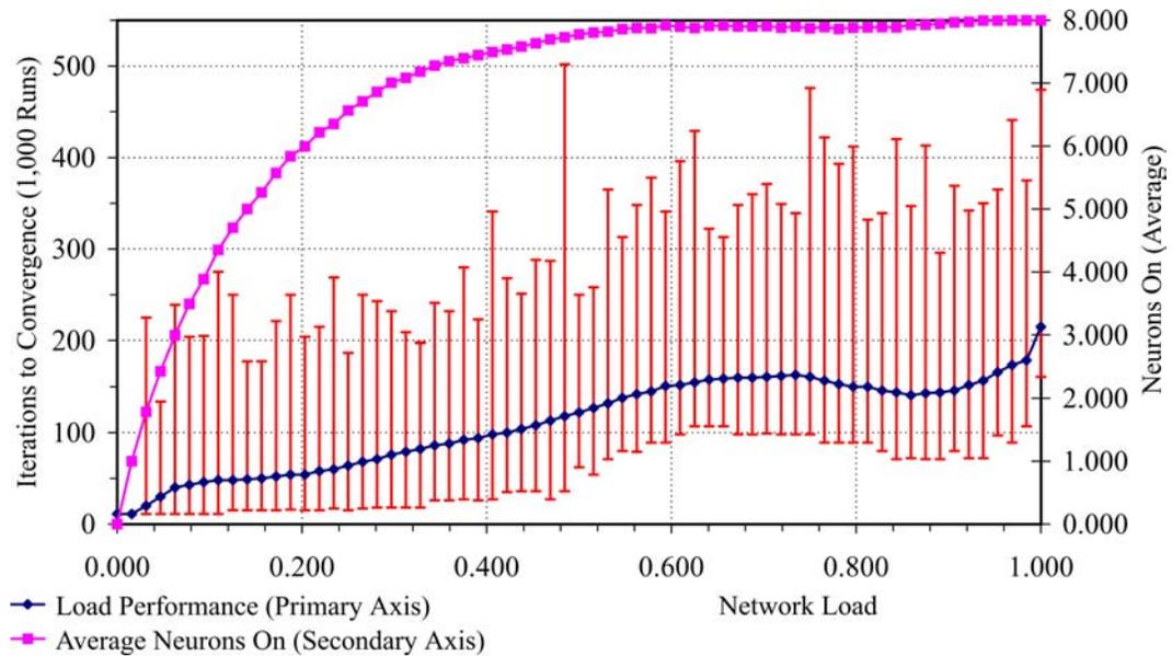
**Figure 68: Effect of Load on Iterations to Convergence with  $Q_{DAC}=1$**
