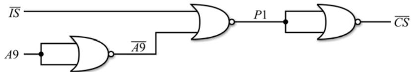
**Figure 92: Chip Select Logic Circuitry**
