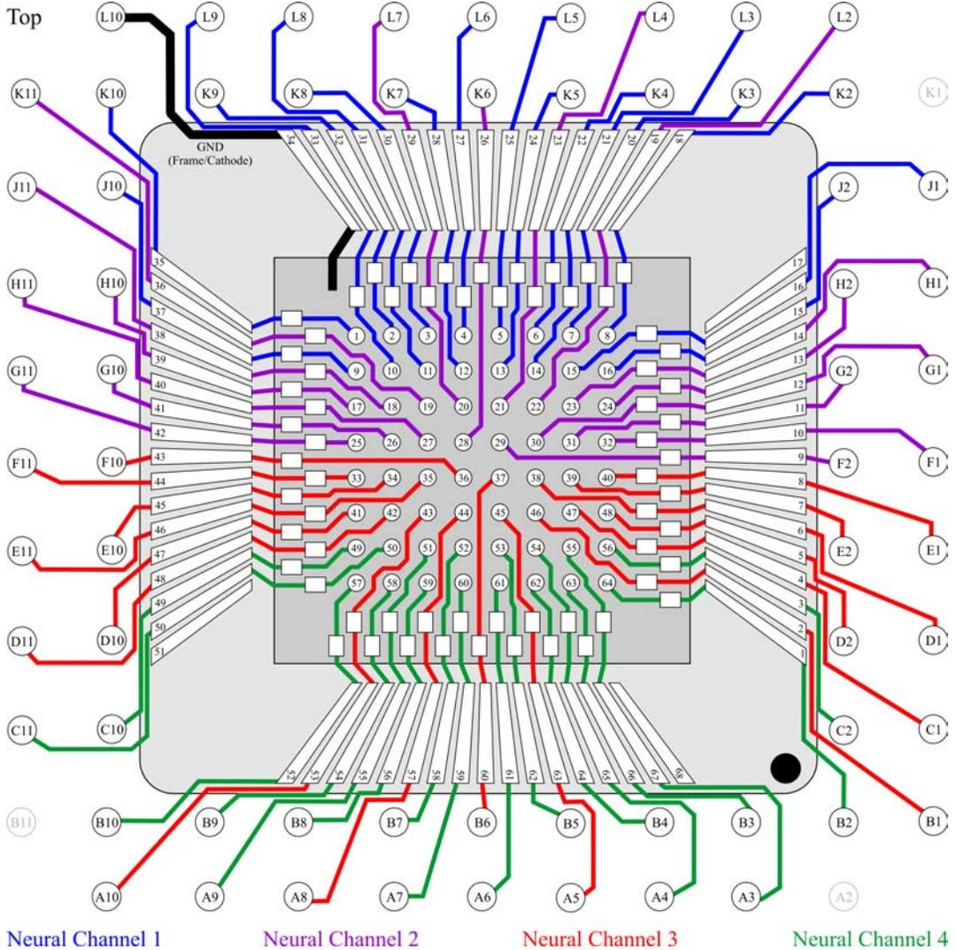
**Figure 104: VCSEL Array Connections**
