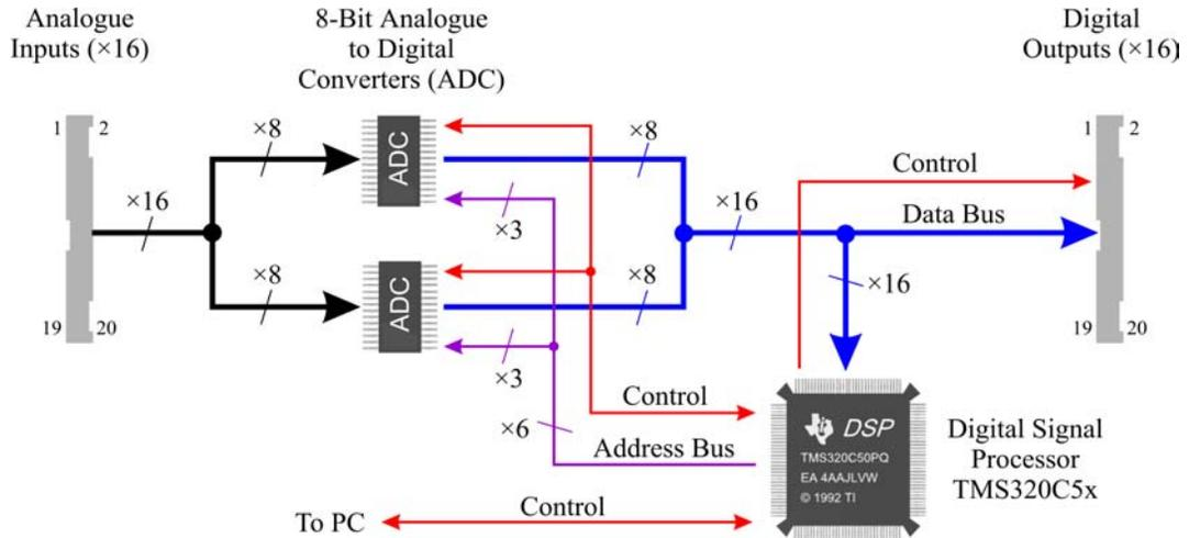
**Figure 89: Digital Signal Processor Module Logical Overview**
