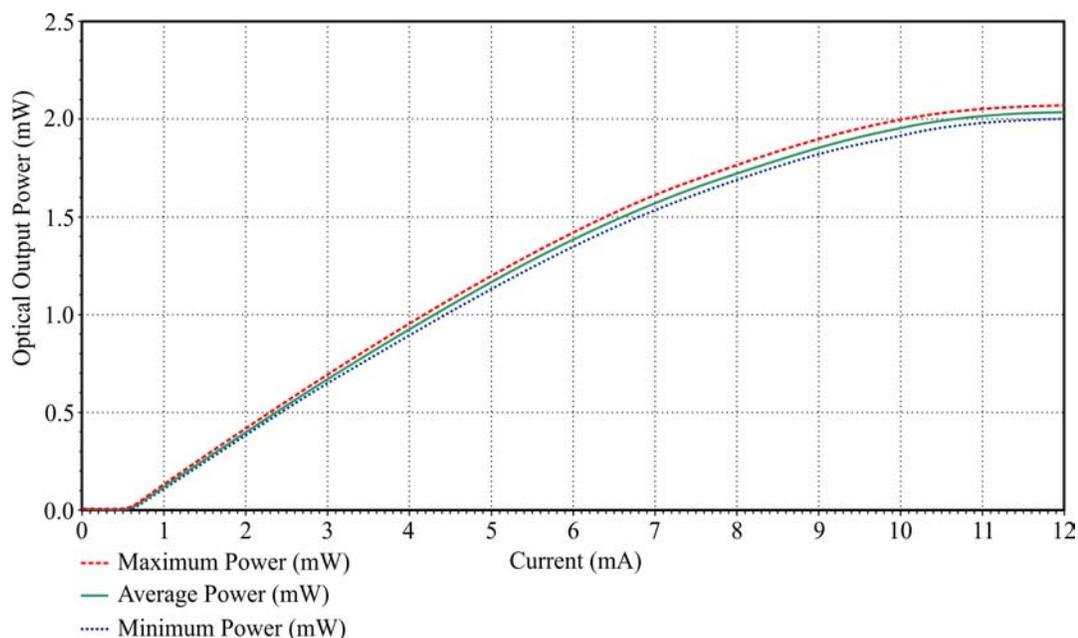
**Figure 109: CSEM D6 VCSEL Optical Output Power Characteristics**
