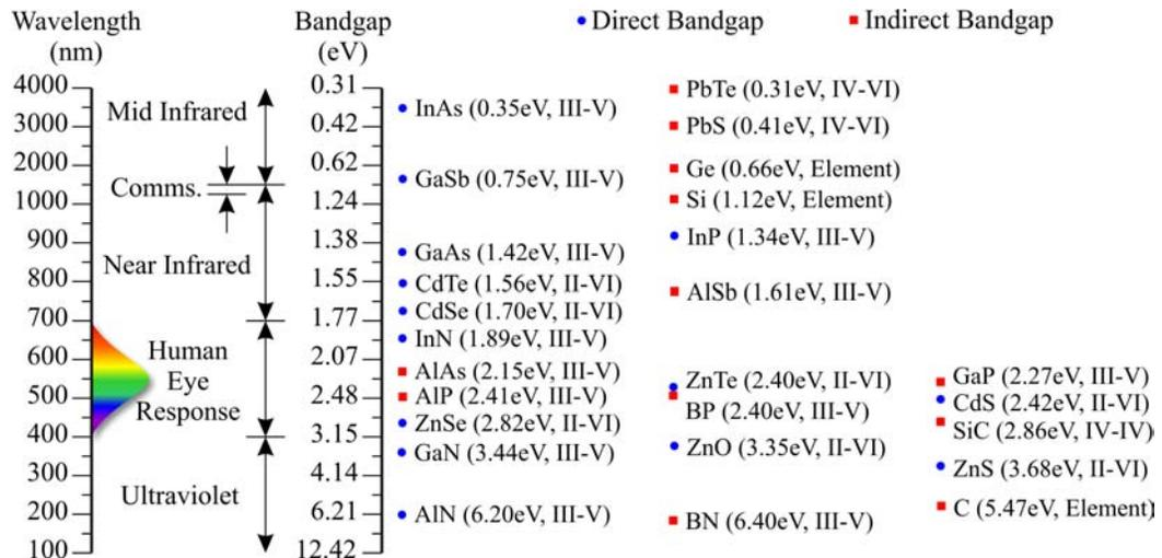
**Figure 25: Bandgap Energies of Elements and Binary Compound Semiconductors**
