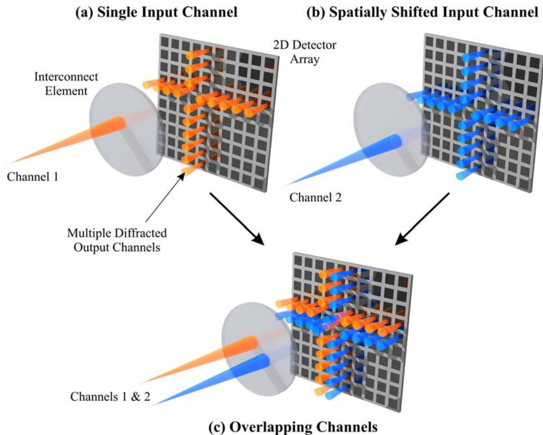
**Figure 8: Manipulating Optical Channels**
