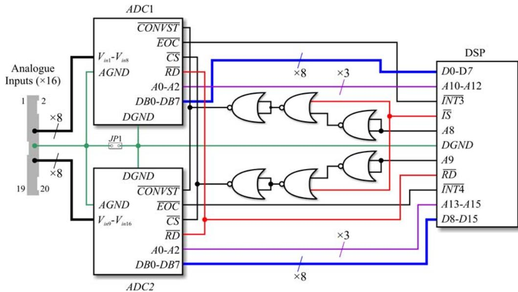
**Figure 93: ADC to DSP Interface Circuitry**
