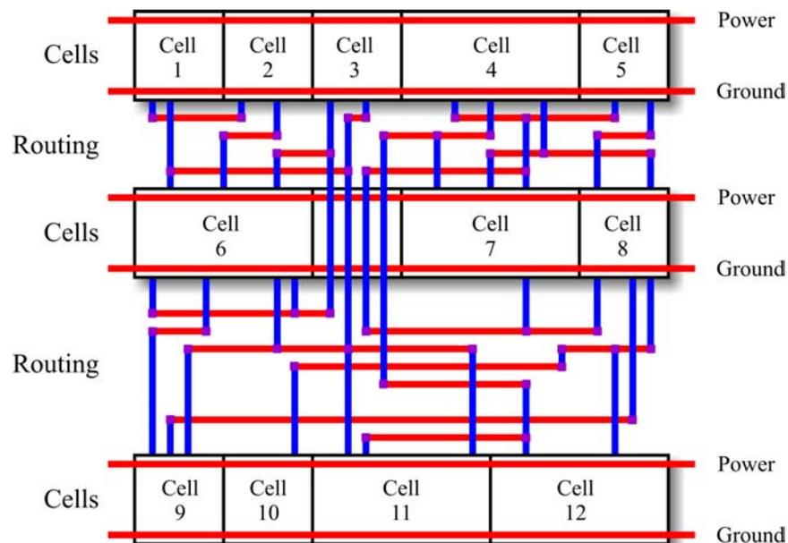
**Figure 122: Standard Cell Layout**
