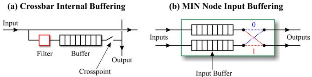
**Figure 22: Switch Internal Buffering**
