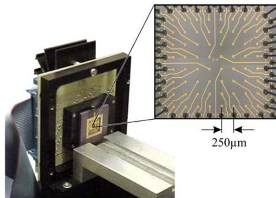
**Figure 103: VCSEL PCB Layout and Mount**
