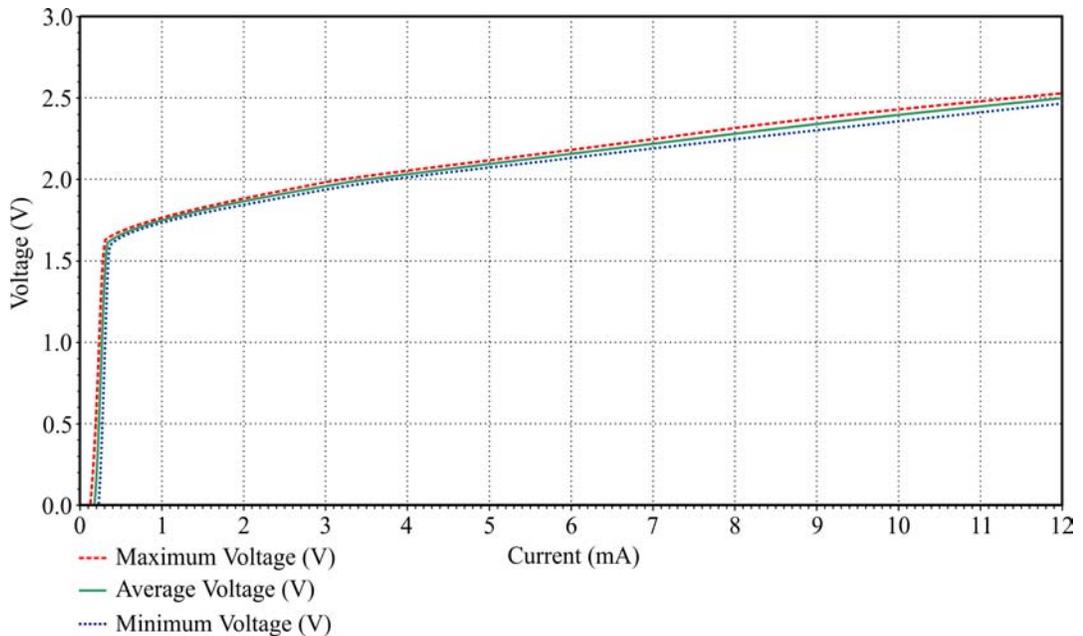
**Figure 74: Lase-Array SN 2640 VCSEL Current to Voltage Characteristics**
