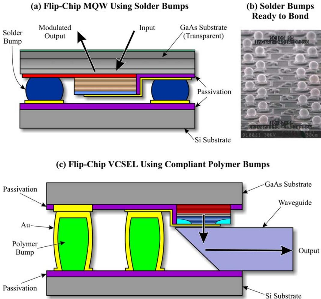
**Figure 42: Flip-Chip Bonding of Incompatible Substrates**
