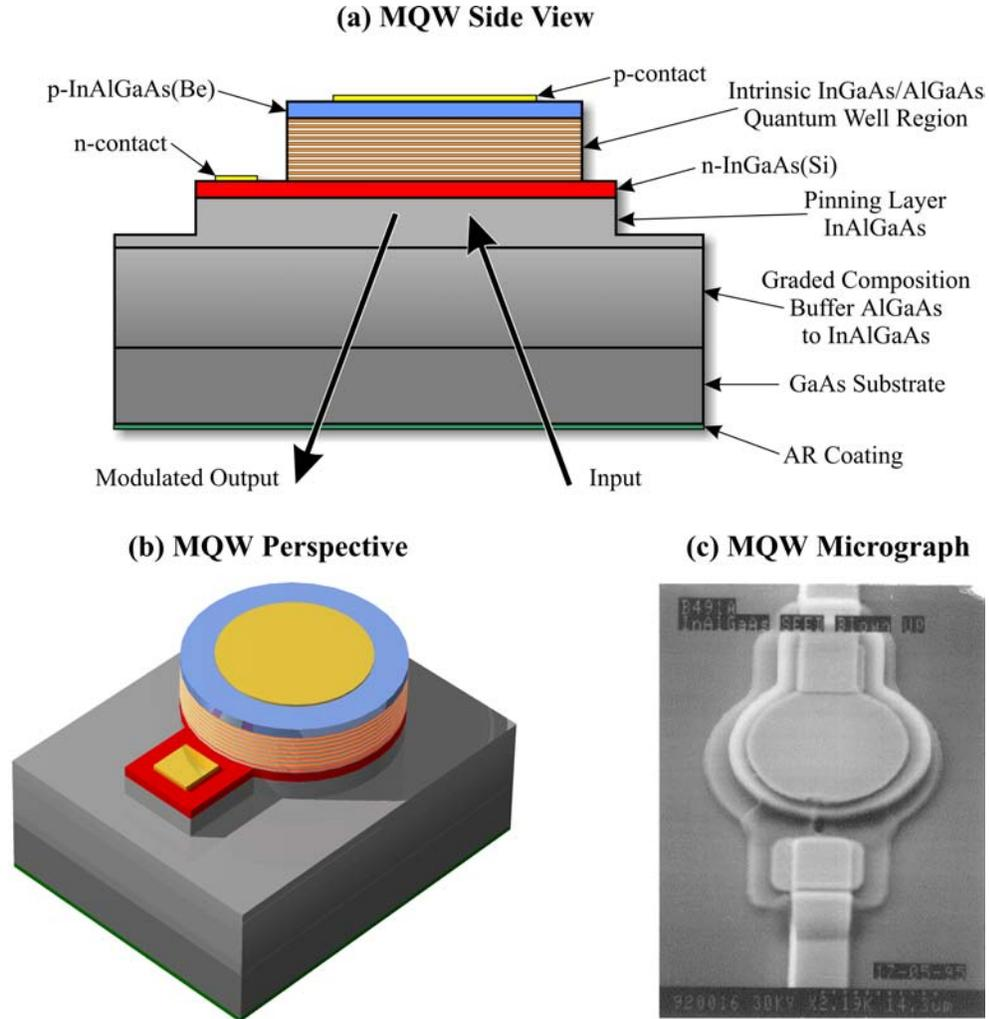
**Figure 29: Multiple Quantum Well (MQW) Modulator**
