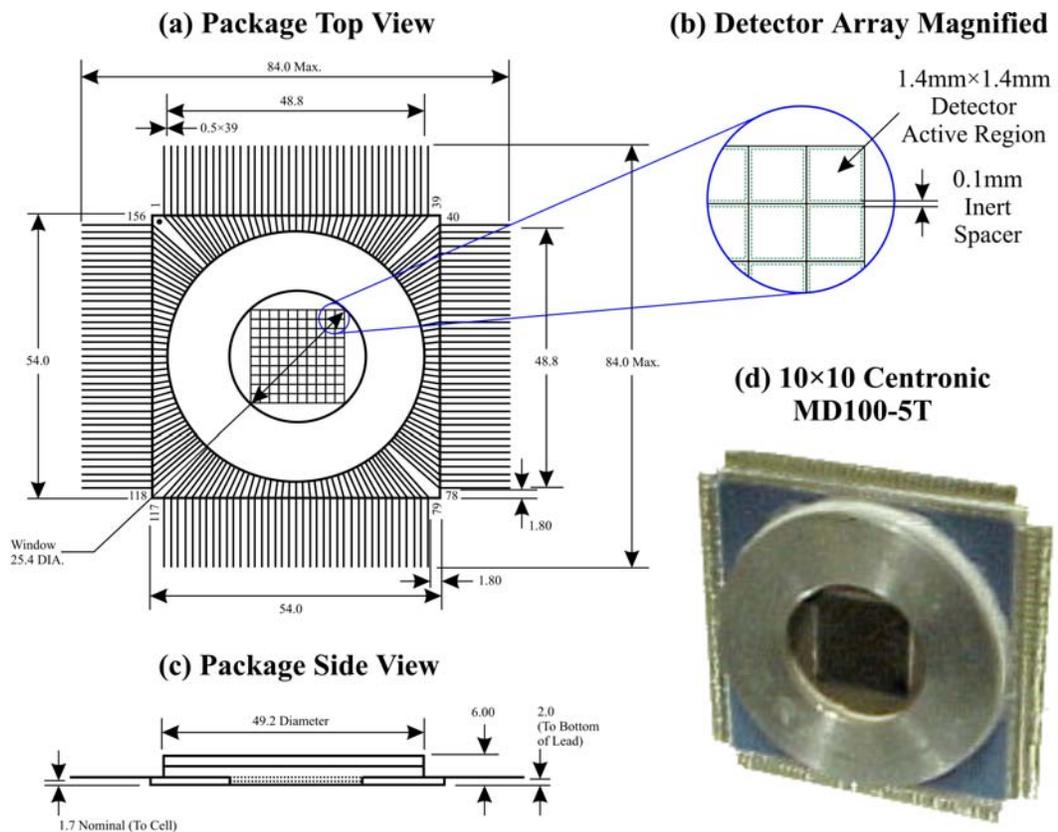
**Figure 80: 10×10 Centronic MD100-5T Photodiode Array**
