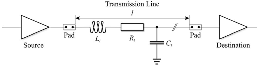
**Figure 3: Electrical Transmission Lines**
