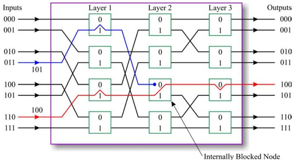
**Figure 20: Banyan Network - A Multistage Interconnection Network**
