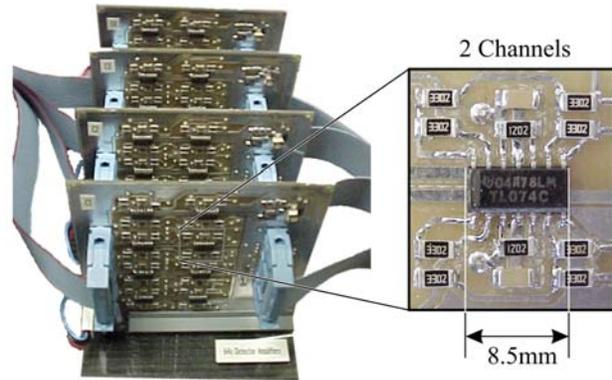
**Figure 115: Transimpedance Amplifier Module PCB Layout and Image**
