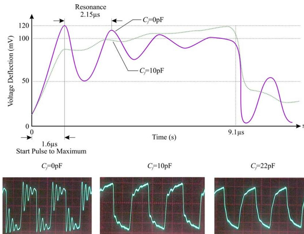
**Figure 117: Transimpedance Amplifier Response and Resonance**
