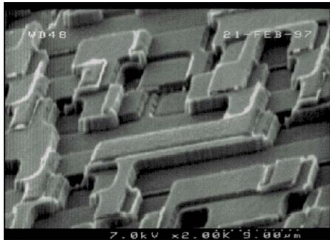
**Figure 36: Multilevel Diffractive Optic Element**
