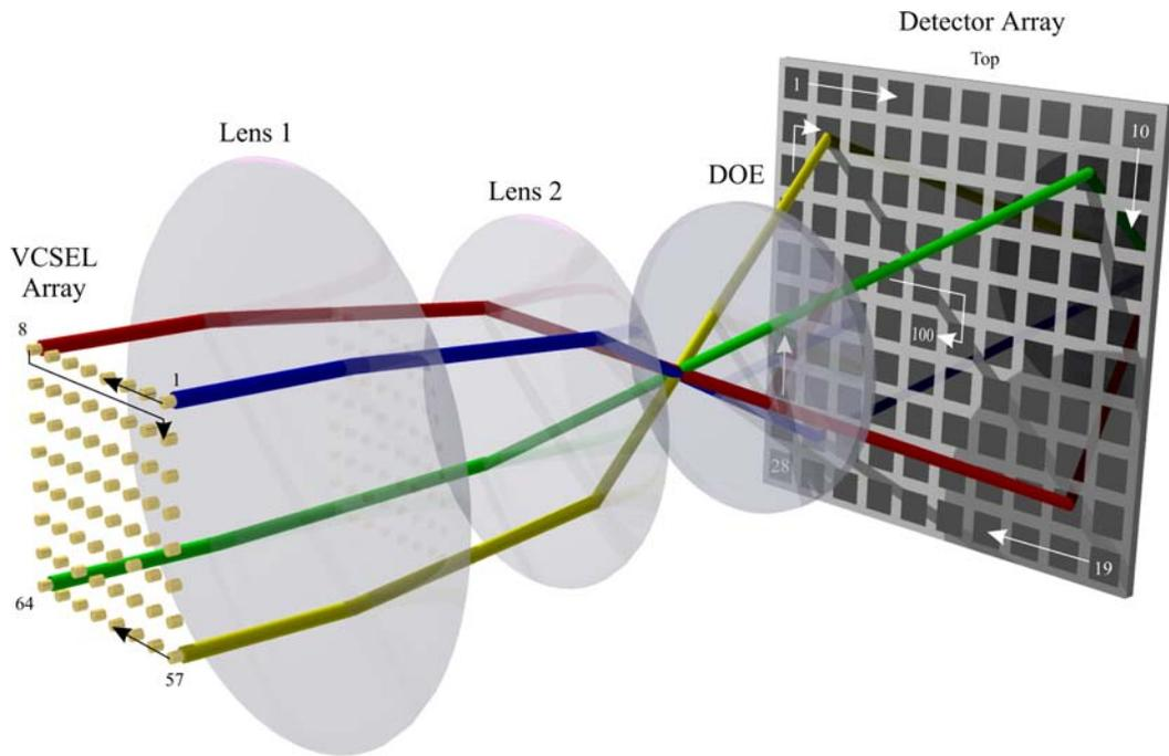
**Figure 105: VCSEL to Detector Mapping**
