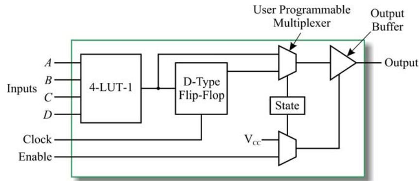
**Figure 124: Configurable Logic Block (CLB)**
