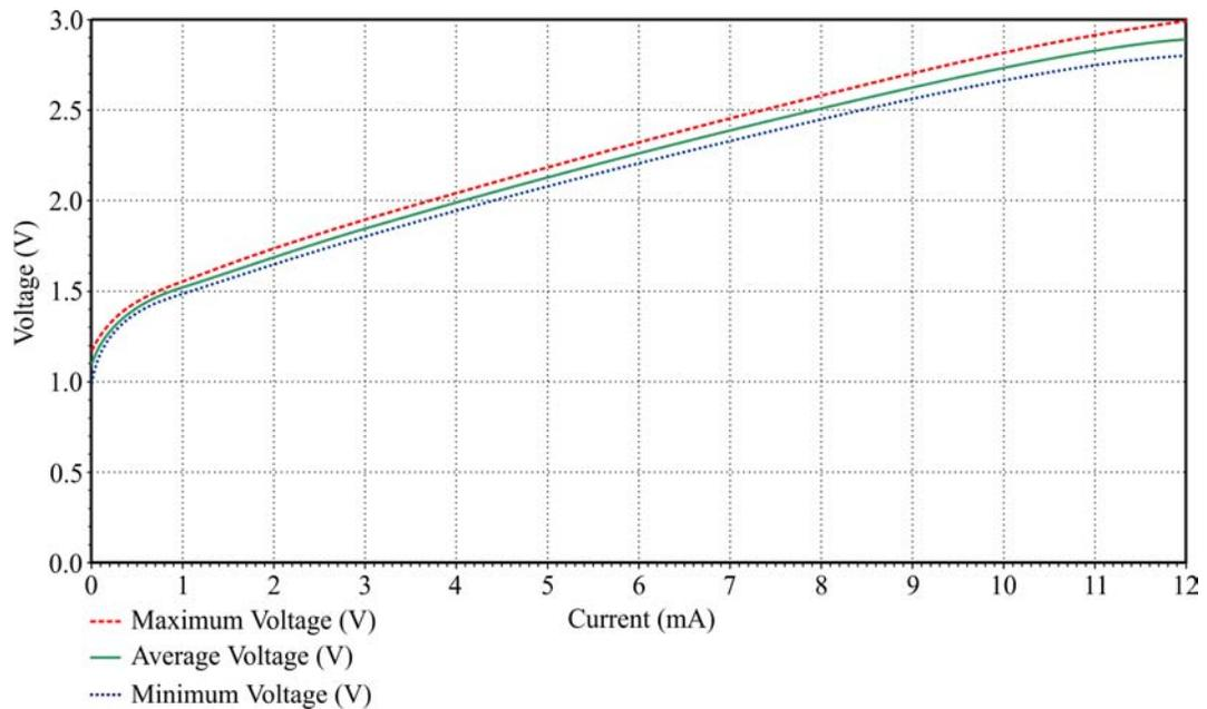
**Figure 108: CSEM D6 VCSEL Current to Voltage Characteristics**
