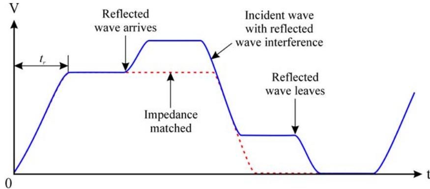
**Figure 5: Reflection in Transmission Lines**
