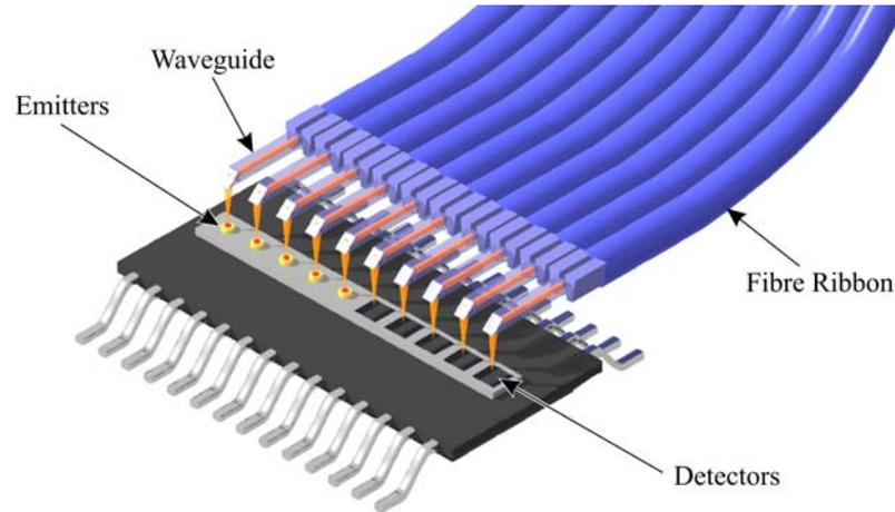
**Figure 39: Fibre Ribbon Interconnect**
