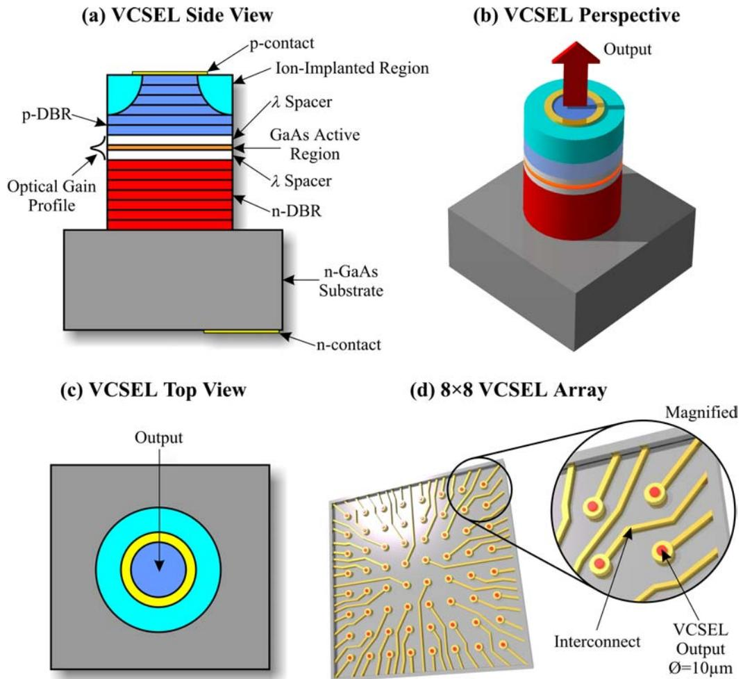
**Figure 28: Vertical Cavity Surface Emitting Laser (VCSEL)**
