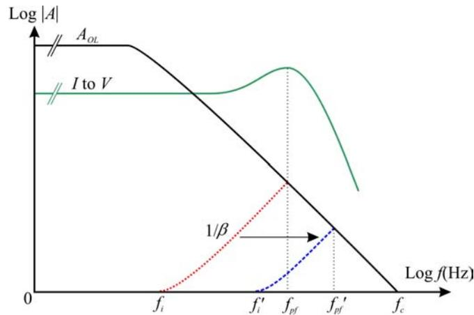
**Figure 35: Transimpedance Amplifier Frequency Response Plot**
