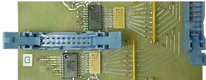
**Figure 99: Digital VCSEL Driver Module Images**
