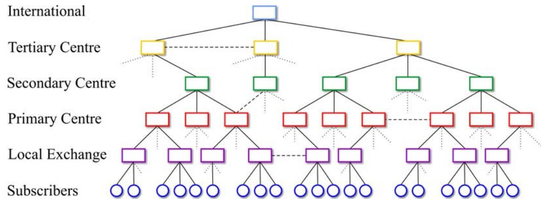
**Figure 14: Hierarchical Routing System**
