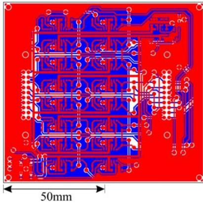
**(b) 4×Transimpedance Amplifier Module Images**
