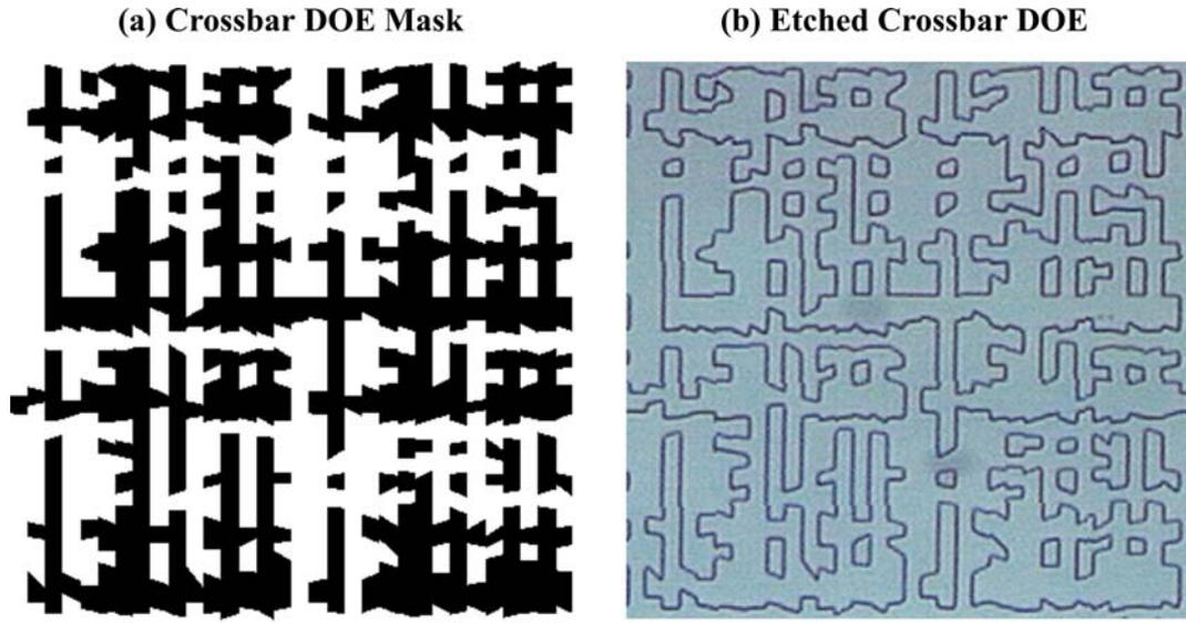
**Figure 77: Diffraction Optic Element Phase Profile**
