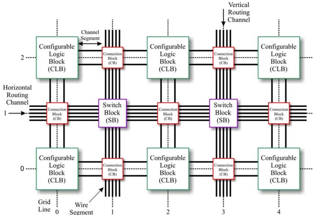
**Figure 125: Symmetrical Array Routing**
