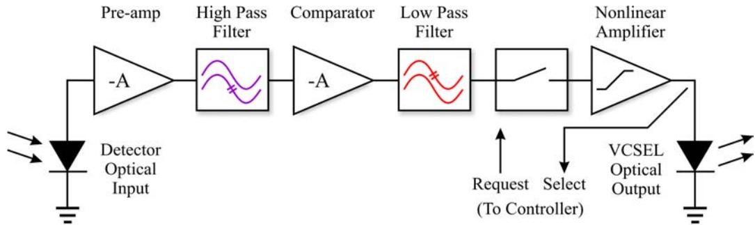
**Figure 58: Single Electronic Channel from the First Generation Neural Network**
