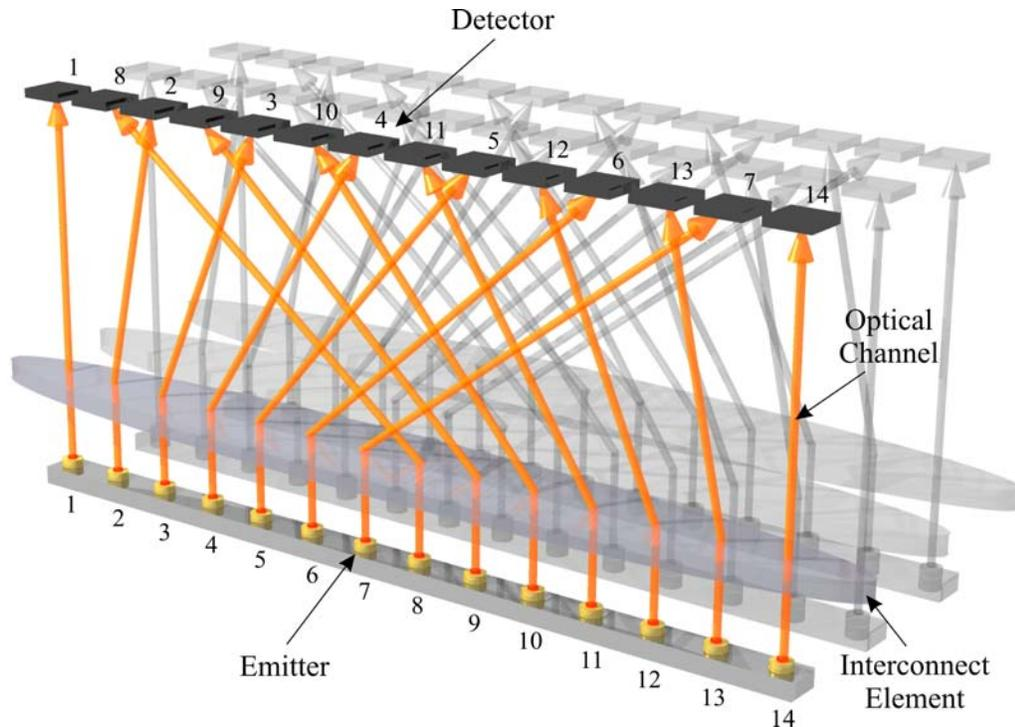
**Figure 11: Optical Implementation of Stone's Perfect Shuffle**
