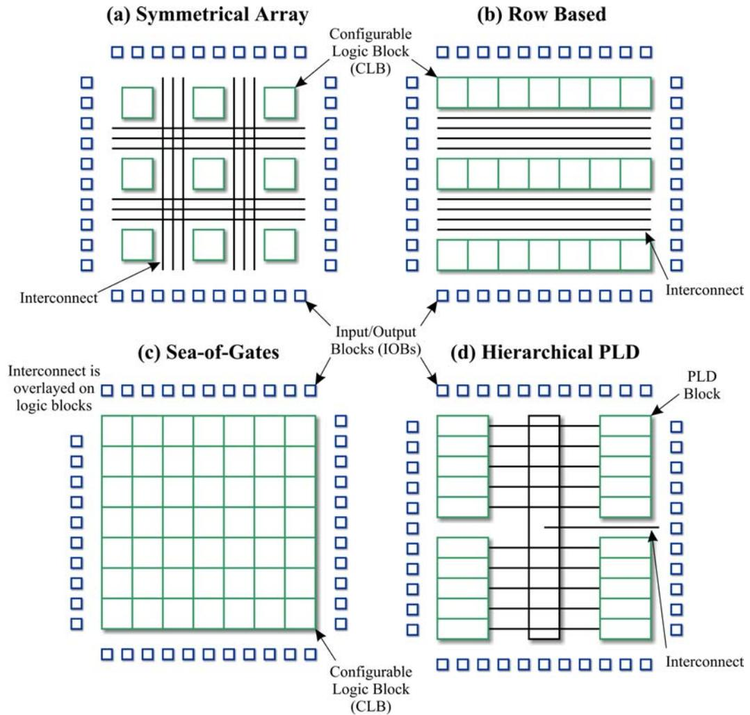
**Figure 123: Main FPGA Classes**
