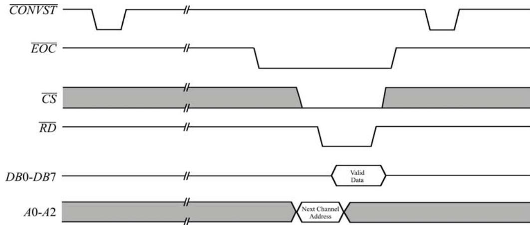
**Figure 90: ADC Conversion Flow and Data Readout**
