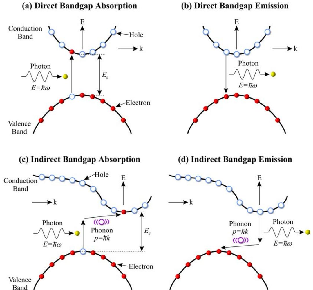
**Figure 24: Direct and Indirect Bandgaps**
