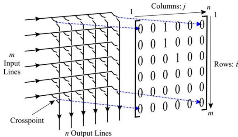
**Figure 52: Matrix Representation of Crossbar Switch**
