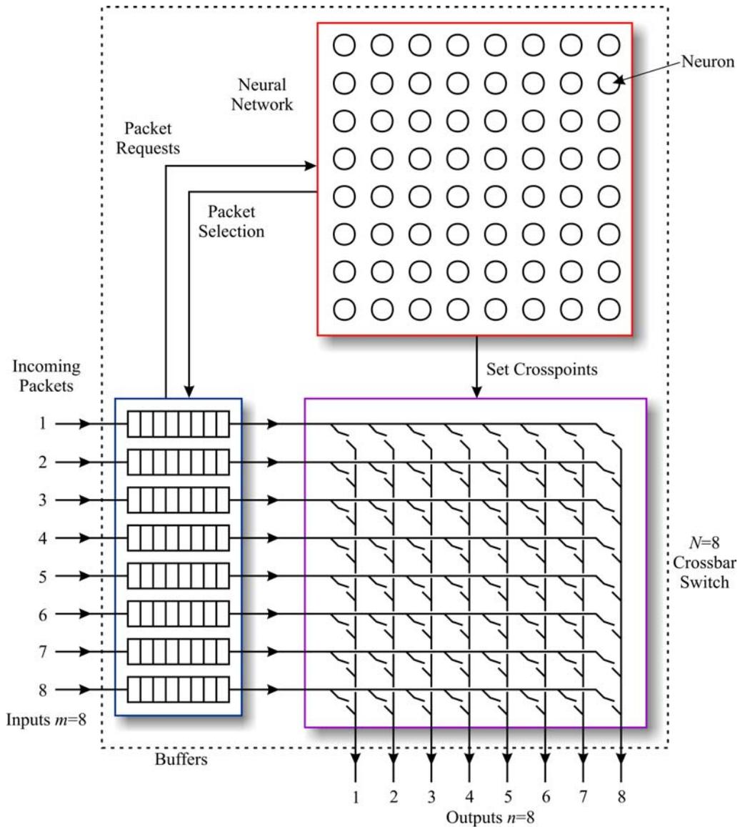
**Figure 50: Neural Network Crossbar Switch Controller**
