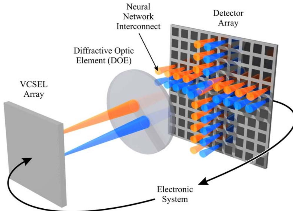
**Figure 54: Neural Network Optical System**
