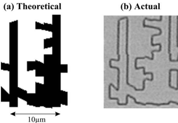
**Figure 55: Photolithographic Transfer Error**
