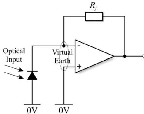
**Figure 33: Unbiased Photodiode Transimpedance Amplifier**
