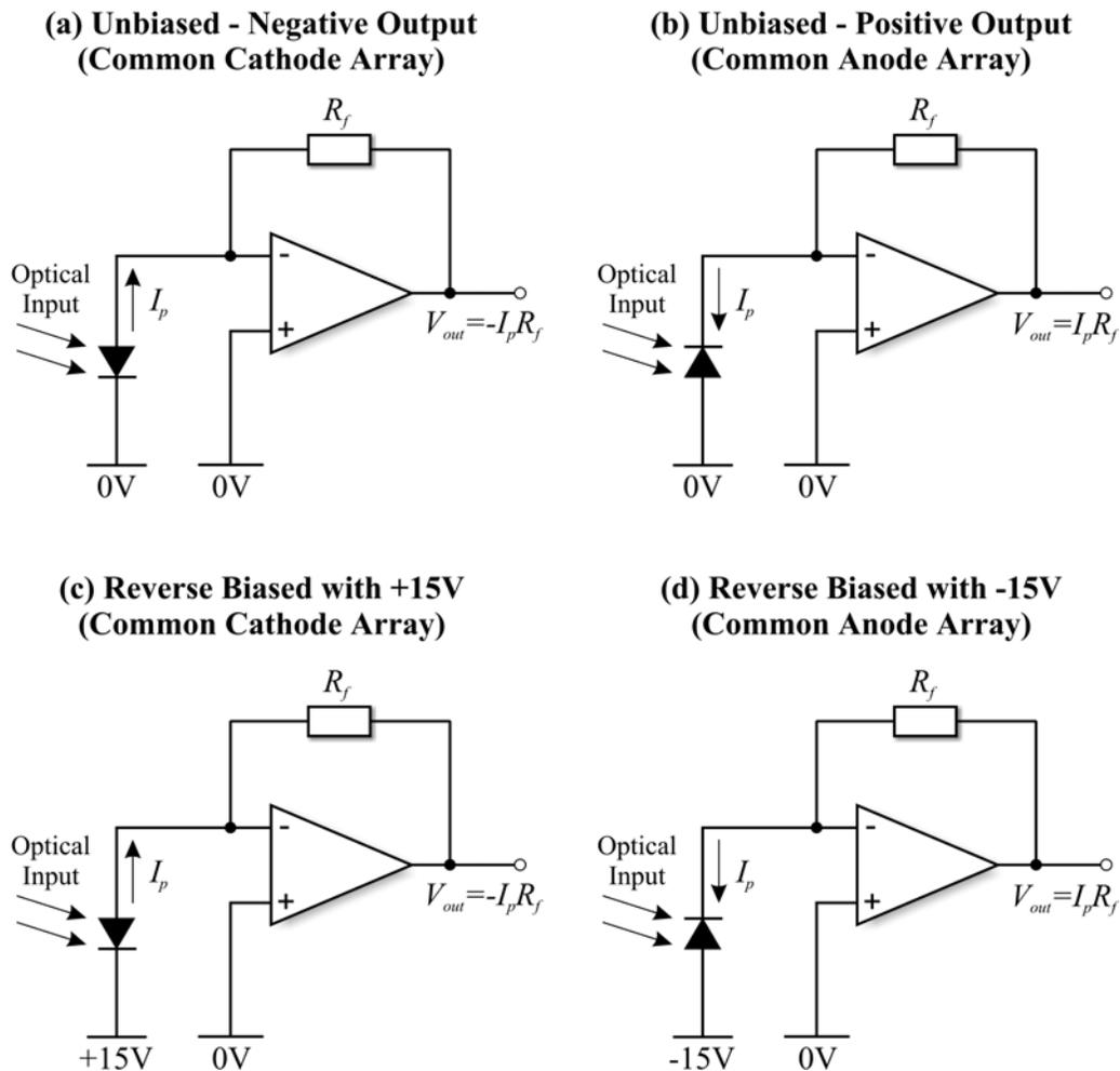
**Figure 32: Photodiode Modes of Operation**
