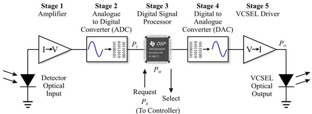
**Figure 59: Single Electronic Channel from the Second Generation Neural Network**
