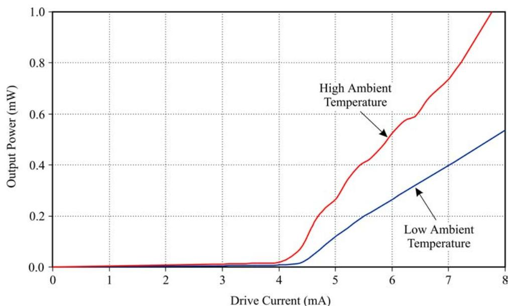
**Figure 75: VCSEL Array Temperature Stability**
