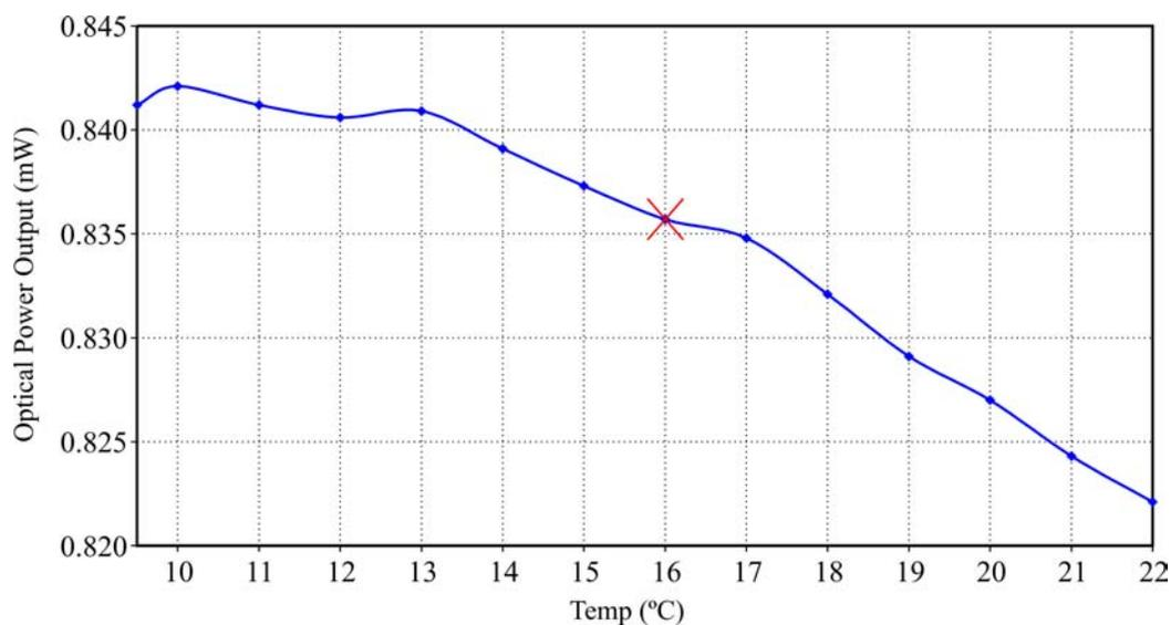
**Figure 111: Temperature Stability of CSEM D6 VCSEL Array**
