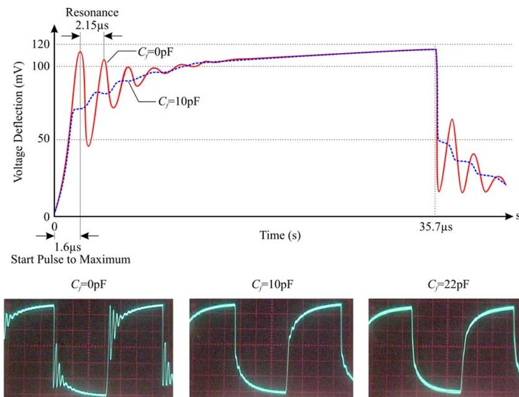
**Figure 116: Transimpedance Amplifier Response and Resonance**
