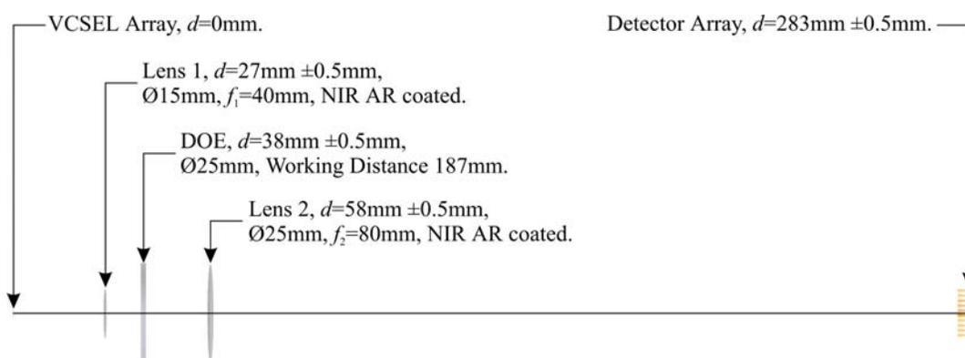
**Figure 72: First Generation Optical System**
