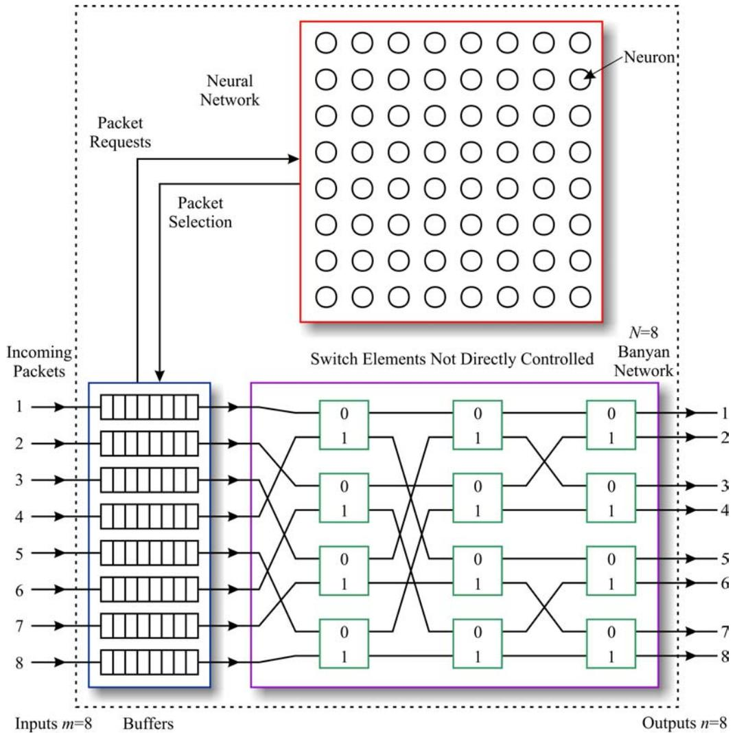
**Figure 51: Neural Network Controller for a Self Routing Multistage Banyan Switch**
