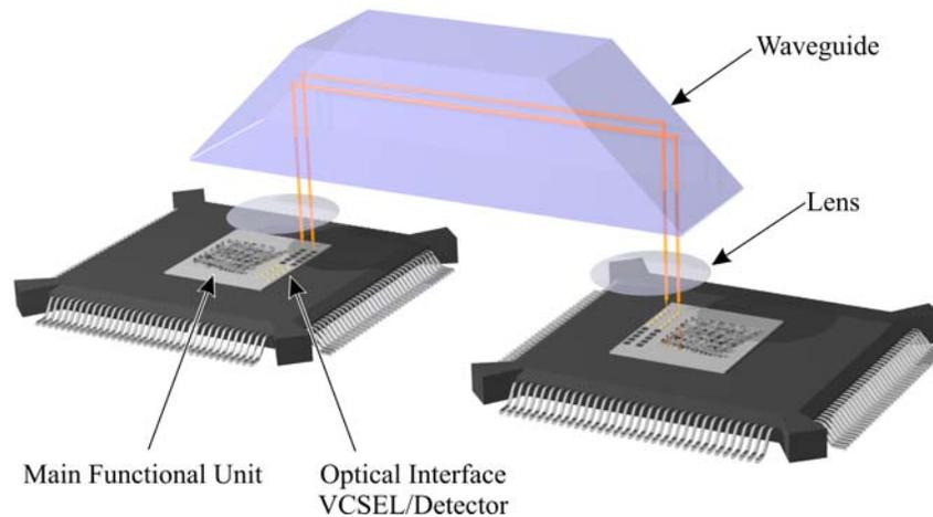
**Figure 41: Chip-to-Chip Interconnect**
