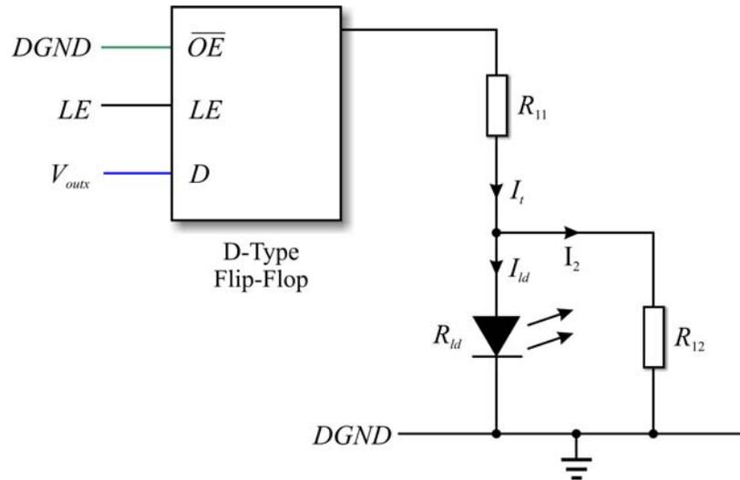
**Figure 97: Digital VCSEL Driver Circuitry**
