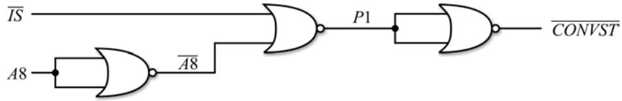
**Figure 91: Conversion Start Logic Circuitry**
