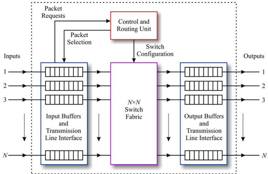
**Figure 18: Packet Switch Architecture Overview**
